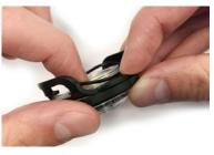
7. Place the o-ring back in its groove<sup>3</sup>.
