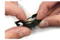
7. Place the o-ring back in its groove.
